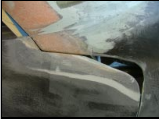
Picture 4, Caption: With the door jamb now complete, door skin spacing needs to be fixed to achieve a uniform gap between door skin and fenders. This corner is the worst case as it has a gap of over an inch.
