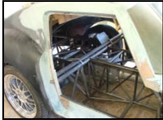
Picture 2, Caption: Door jamb with completed weather seal mounting flanges. The door was put on and taken off at least a half dozen times to check seal placement and overall fitment.
