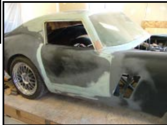
Picture 6, Caption: Body filler is used around the rest of the door skin to achieve a uniform 3/16 inch gap.
