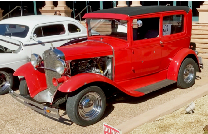
Al Hoesner owns this steel bodied 1931 Ford Model A 2-dr sedan. it's powered by a 283 V-8 and has a 350 auto tranny.
