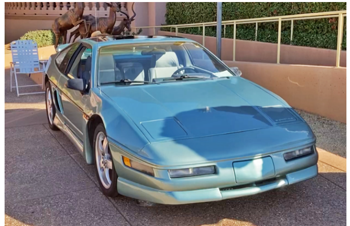
Jim Wagner built this car from a 1986 Pontiac Fiero by replacing body panels to turn it into a Corvette look-alike. A mid-engine V-6 provides the power.
