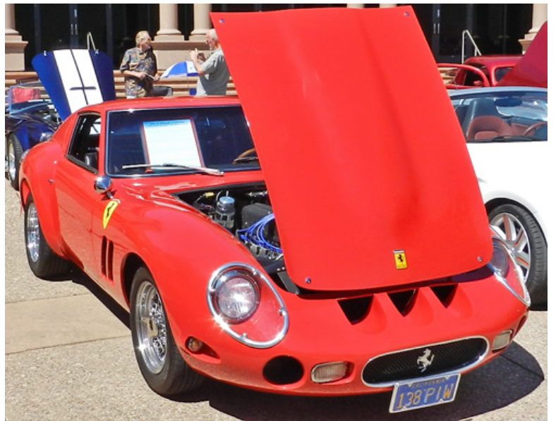
Mike & Melinda Koken drove their Ferrari 250 GTO replica from Southern California to our show. It is an Alpha 1 GTO kit powered by a 2.6 L Nissan OHC engine
