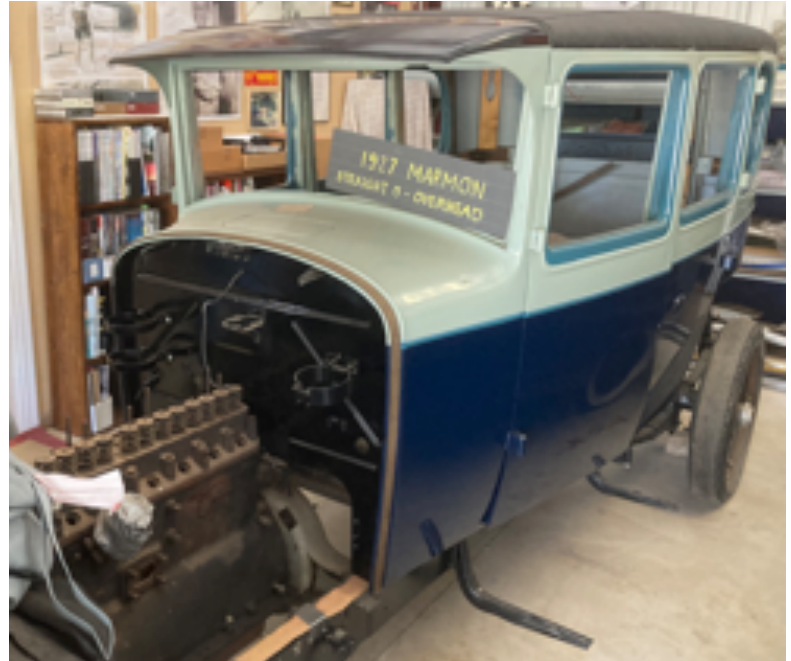
1927 Marmon - 8-cylinder OHV engine (below)
