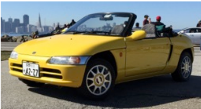
Below: Honda Beat is a mid-engined 2-seater produced from '91 to '96. Total cars produced was around 33,600. Engine was 656 cc, 63 H.P.
