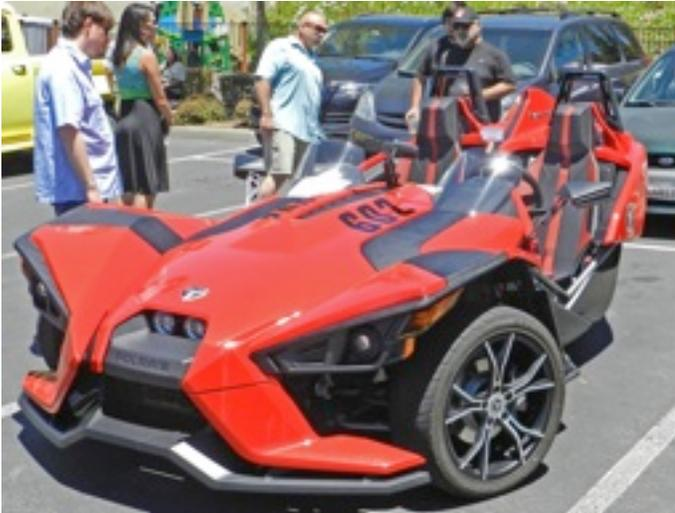
An unusual 3-wheeler that I haven't seen before was a Polaris Slingshot. It was a front engine, rear drive (single wheel) vehicle that the owner told me was a real 'autocross' contender. It was powered by a 2.4 liter, 4-cylinder GM Ecotec engine that claimed about 173 HP output. There were lots of late model cars including Corvettes and Porsches and a fair number of Macho 4-WD off-road machines plus the custom shown below.
