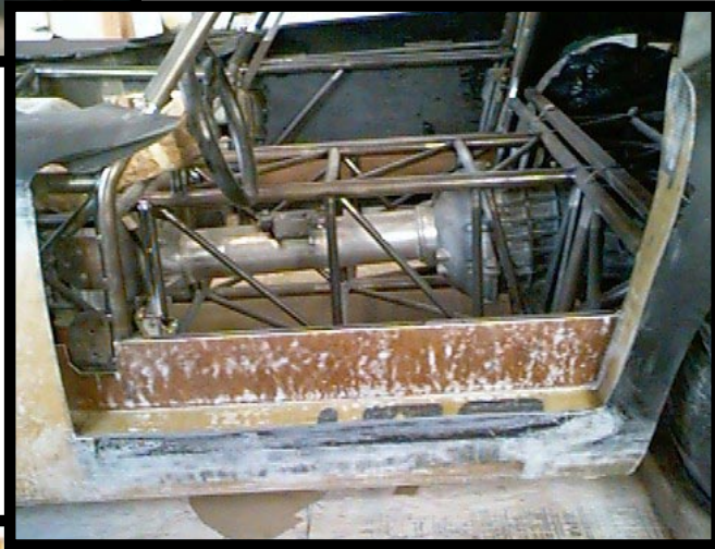
Shown below:: The lower door opening is formed by pop riveting a piece of fiberglass in place and then filling the remainder of the space with foam. The edges have been ground to a taper and gel coat roughed up in preparation for fiberglassing over the foam.
