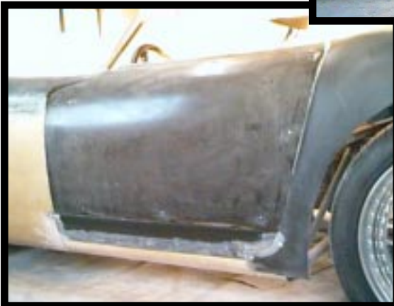
Shown below:: The lower door opening is formed by pop riveting a piece of fiberglass in place and then filling the remainder of the space with foam. The edges have been ground to a taper and gel coat roughed up in preparation for fiberglassing over the foam.
