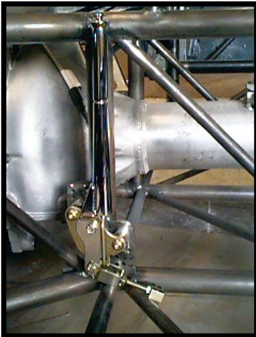
Above: The hand brake lever mounts to the chassis with a couple of bolts. The lever has an adjustable cable block for attaching the cables and adjusting slack from them.
