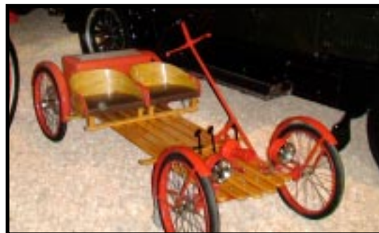
Below: 1928 Auto-Red-Bug. 12 volt electric power from two car batteries. Cost $325
