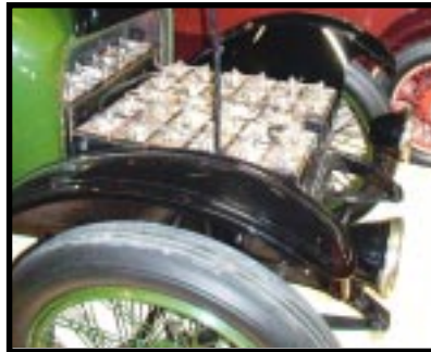
Above: 1914 Detroit Electric with front battery pack at left.
