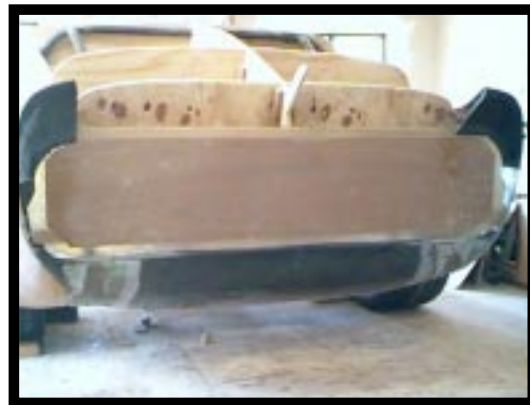
Below: A new fiberglass piece was built from scratch to fill the Kamm-back portion of the rear body work.
